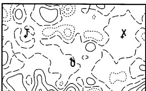
FIG. 4. Difference Fourier sections passing through the T, X, and O sites. Plot details are as described in the legend for Fig. 3.
